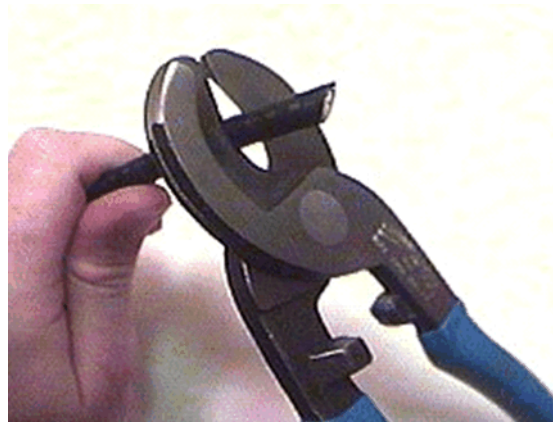
Figure C-1. Coax Cable Cutting Technique
