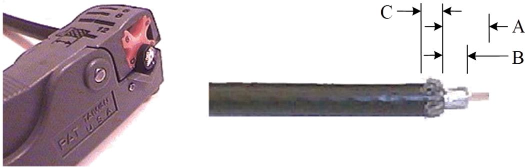
Figure C-2. Cutting Technique for Removing Foil in the Braid
